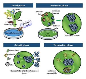
example, glutamic and aspartic acids on the surface of yeast or the reductase enzyme in the cytosol of fungi reduce metal ions to form nanoparticles.
